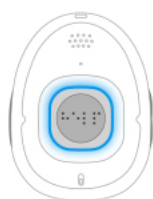
Battery is Charged
